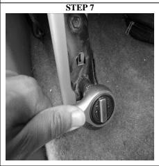
**Rear Bench**. Lift up the 60/40 rear bench seats and remove (5x) 12mm bolts to release bench from vehicle.
