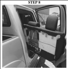
**Rear Bench.** Firmly lift the bench, remove from the vehicle & place in a clean area to continue with the fitment of the seat covers.
